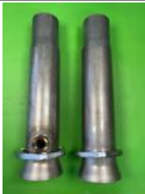
2.5"Ball Header to 2.25"OD 12"Long 409 Stainless 3 Bolt Socket Reducer W/O2 Bung
