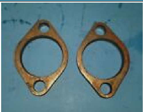
2 1/8" ID 2 Bolt Slip On Formed Steel Flange 3 1/8" Bolt Center 3/8" Thick
