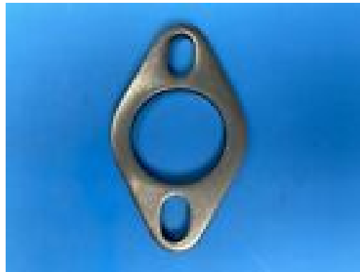
2.05" Header Collector Rings Weld-Slip On 2 Bolt Steel Flange 3.5"center line
