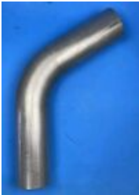
3"60 Degree 14 Gauge Aluminized OD/OD Mandrel Bend Elbow Exhaust Tubing Pipe
